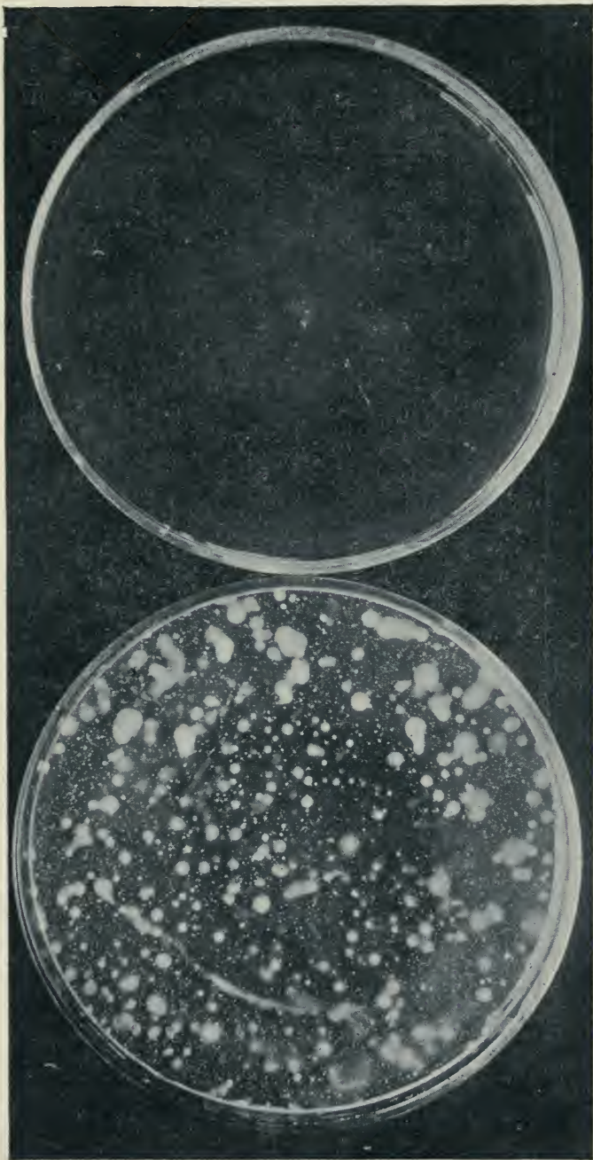
PETRI PLATES ILLUSTRATING THE EFFICACY OF PASTEURIZATION AT 68° C. FOR THIRTY MINUTES IN DESTROYING THE BACTERIA OF MILK.
